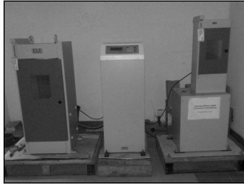
Figure 7: Compressive strength test machine Figure 8: UTM machine
