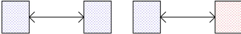
**Enclosure** - distance from the inside of the edge of a shape to the outside of the edge of another shape.
