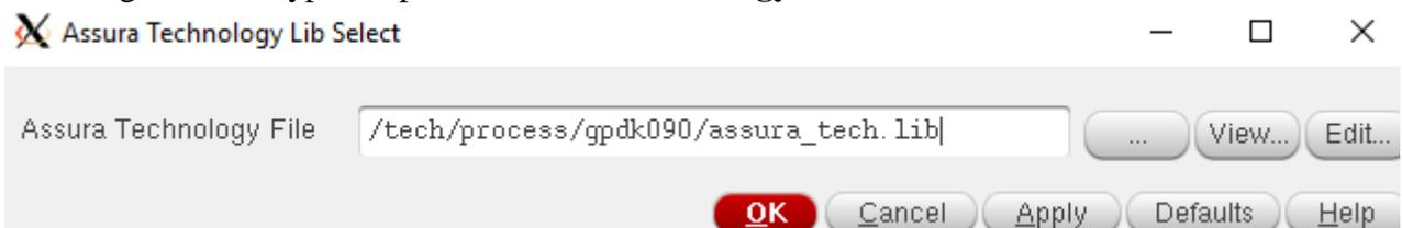
2. Execute *Assura* → *Run DRC*. A DRC window appears as shown below. Fill the form as indicated in the picture.
